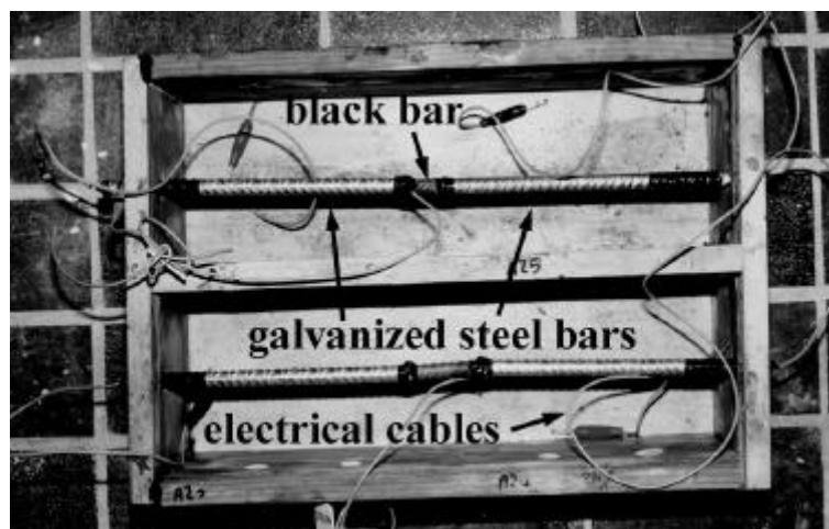
Fig.1. Two assembled bars with Sa/Sc=20 (top) and Sa/Sc =7.5 (bottom), used to study the galvanic protection on discontinuities.
