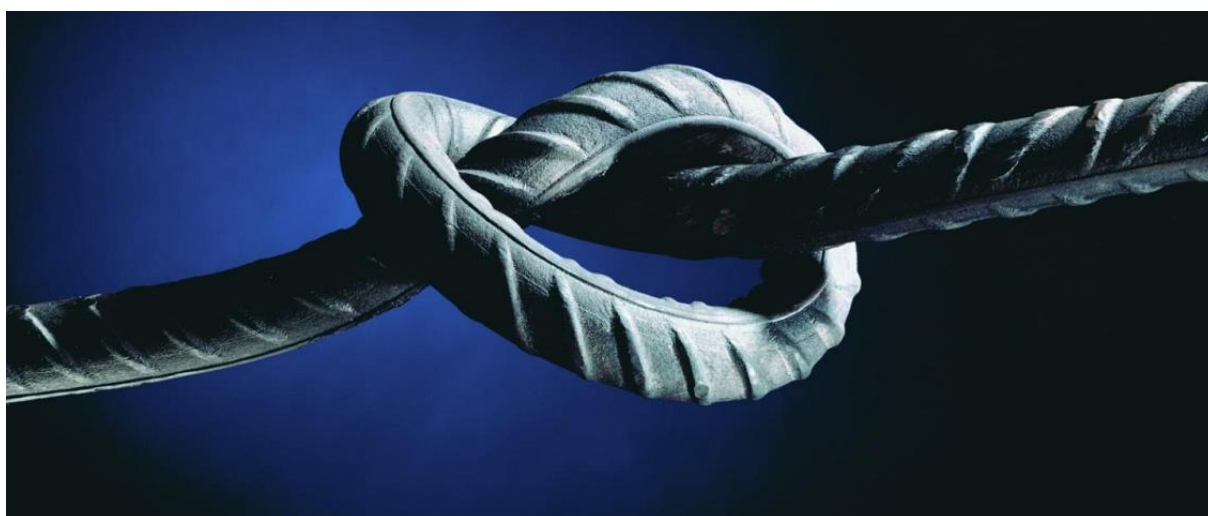
Knot with cold-drawn steel deformed bars for concrete reinforcement, diameter Ø 28 mm
