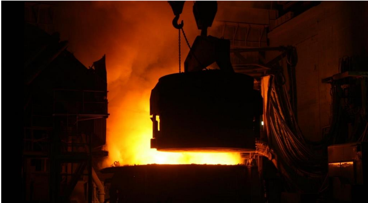
Steel scrap loading into the smelting furnace
